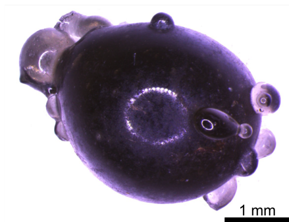
Figure 1.4: Optical micrograph of agglomerated objects adhered to the exterior of sample FLD14, a piece of aerodynamic glassy fallout studied in this dissertation. The bright, circular feature in the center of FLD14 is an artifact of the reflection of the ring light from the optical microscope, highlighting the symmetry of the sample.
